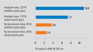
The UV power comparison relates to lamps with the same illuminated length of  $800\ \mathrm{mm}$  and the same tube diameter of  $15\ \mathrm{mm}$
