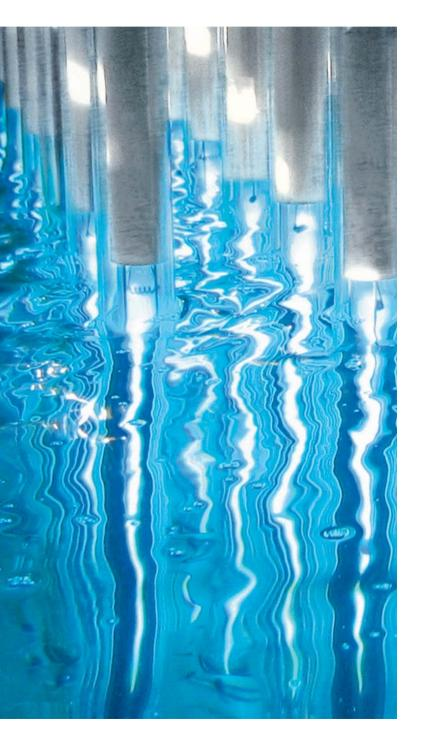
Classical low pressure UV lamps offer exceptional efficiency. 40% of the electrical power can be used for disinfection as UVC radiation at 254 nm. If synthetic quartz glass is used as the lamp material, UV radiation at 185 nm is also emitted for oxidation processes.
